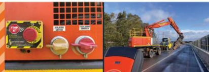
Thompson Safety Stop It - remote E-Stop system installed on a project excavator (left). Spotter's remote activation of E-Stop system simulating control of traffic (right).
